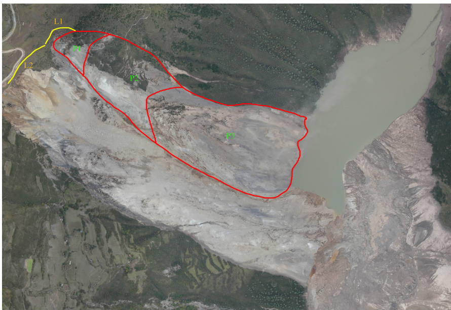
图 7 滑坡后缘裂缝与潜在不稳定斜坡图 Fig.7 Fractures at the trailing edge and the potential unstable slope diagram at Baige landslide
