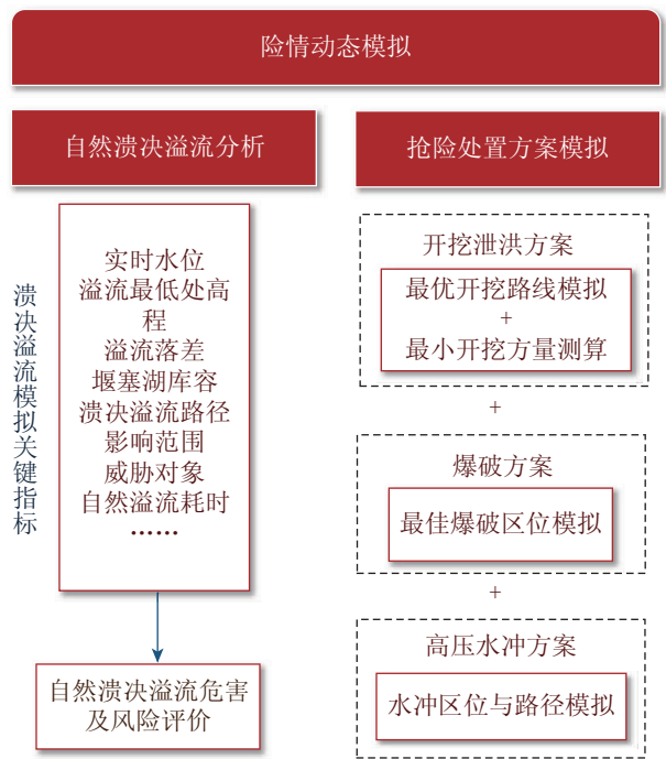
图3 面向滑坡—堰塞湖灾害链的险情动态模拟 Fig. 3 Schematic diagram for simulation of landslide-barrier lake disaster
