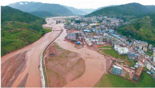
图 7 抬高后的河床使得喜德县城洪水泛滥 Fig. 7 Xide city threatened by uplifted beds and flood
