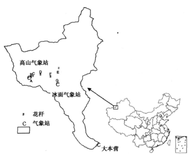
图 1 科其喀尔巴西冰川气象站和冰面花杆分布示意图 Fig. 1 Meteorological stations and ablation stakes on the Keqicabaxi Glacier
