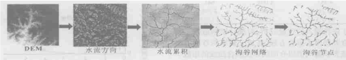
图 1 沟谷网络节点提取示意图 Fig. 1 The graph of extraction of channel network nodes
