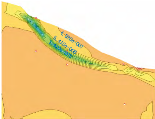
图 9 地震动作用下应变分布特征 Fig. 9 The feature of shear strain under earthquake
