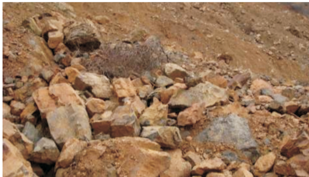
图 9 短程碰撞骤停区 Fig. 9 Area of short-runout collision to arrest
